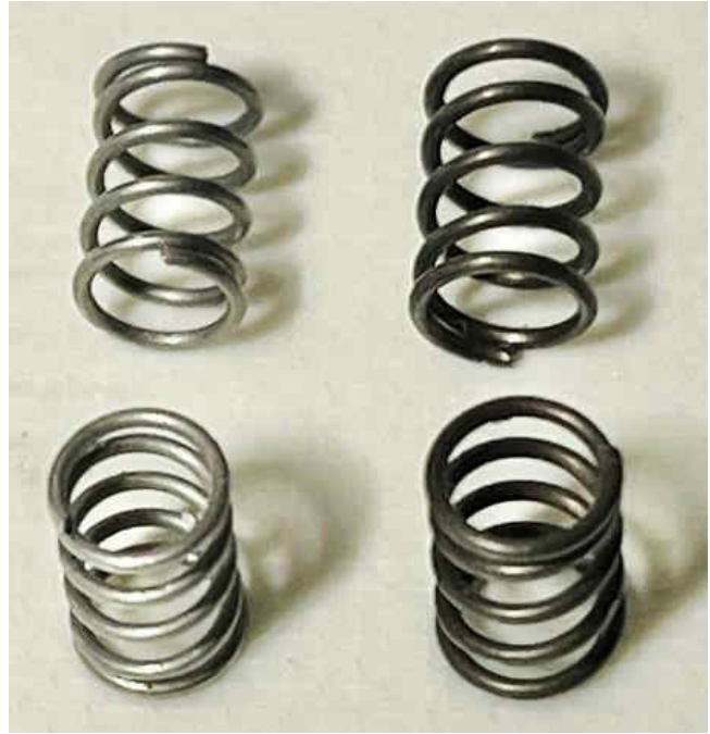
Original springs on left (silver) & new springs on right (black)
