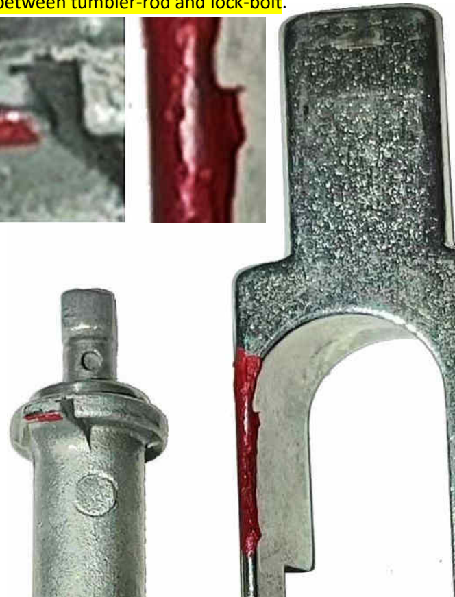
Paint transfer between tumbler-rod and lock-bolt.
