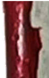
Paint transfer between tumbler-rod and lock-bolt.
